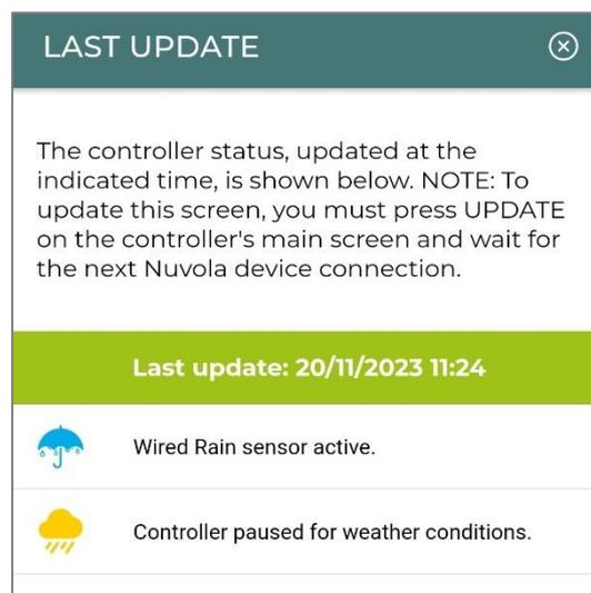
Once the day of pause is over, the controller will automatically exit the pause and return to watering following the automatic programming.
